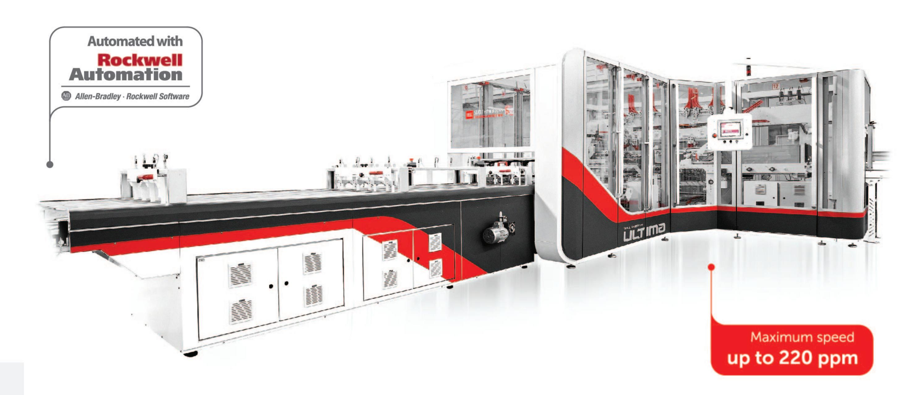
**ULTIMA** is a new generation wrapper with highest production speed on the market and 40% less energy consumption comparing to known conventional models which declare same or similar speed. ULTIMA is the first machine on the market using iTRAK which allows to maintain perfect shape of the packs, even when running at speeds above 200 packs/min, at the same time granting extremely easy and fast changeover time. This supreme and impressive wrapper is undoubtedly a revolution in tissue packaging!
