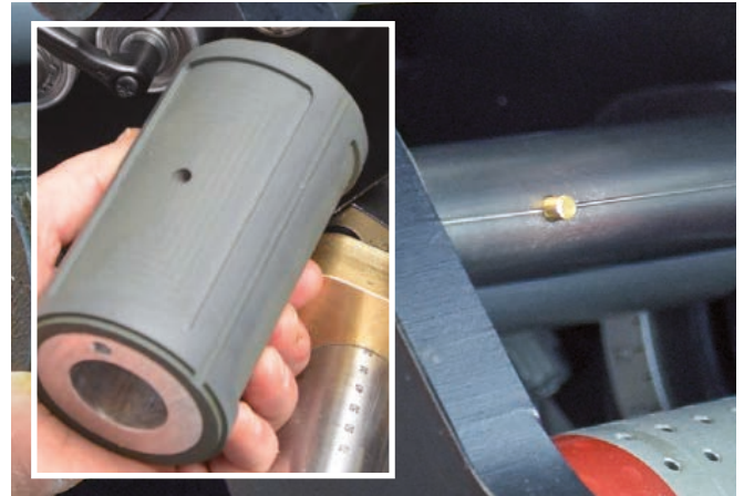
Toolless positioning of the window gummer by means of a PIN system
