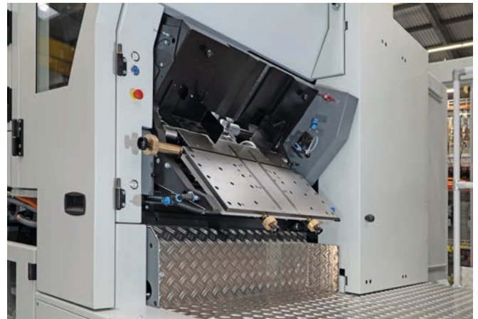
Feed table in parking position. Envelope converting from web.
