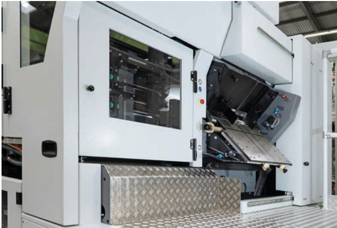
Feed table in working position, Envelope converting from blanks
