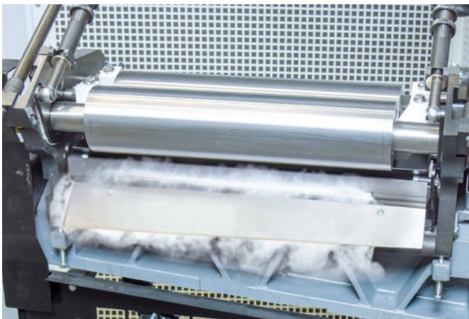
Seal-flap gumming section with glue humidification
