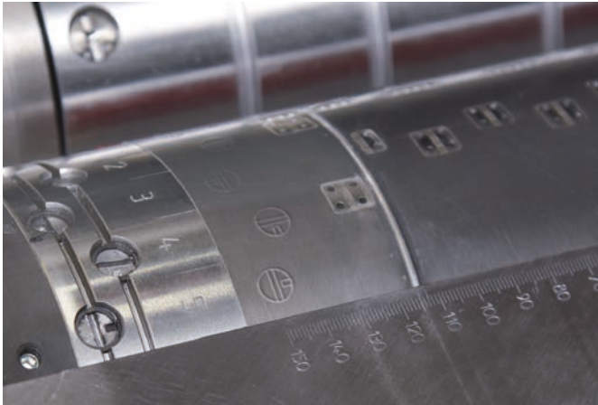
Marked valve positions on the EasyCut® flex die allow quick and easy changeovers
