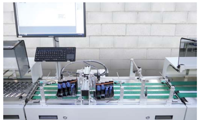
Mail table for inline, end of line read-write personalization.
