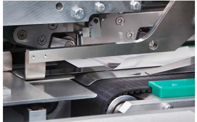
Inserts placed on envelope blank and plough folding of side seams
