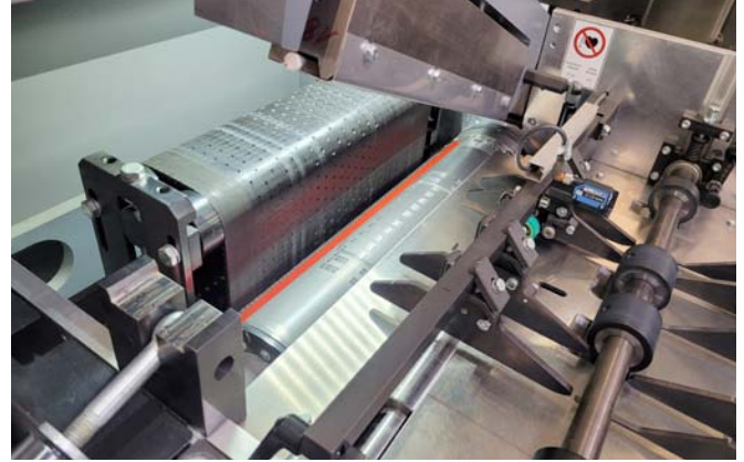
Complete cut using foil knife on magnetic cylinder, vertical vacuum transport
