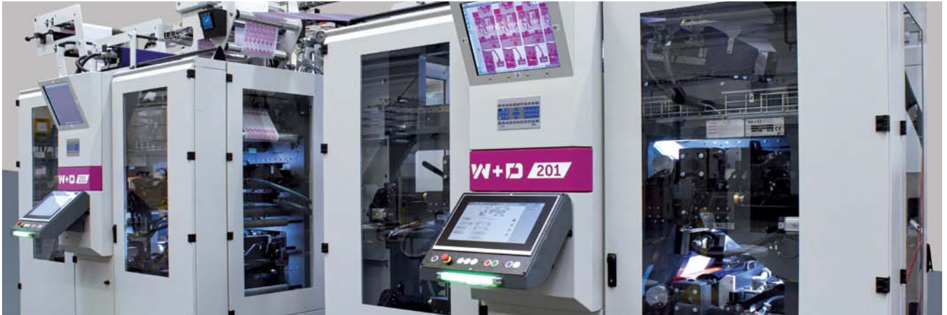
Two W+D 201 Inline-Flexo-print-systems as tandem-combination for production of superior applications
